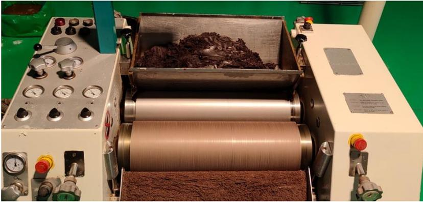
**Figure 3.** Pilot scale refiner
